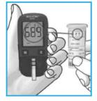
Put the code chip that comes out of the device test strip in its place in the device (this step is not required for devices that do not need coding).
