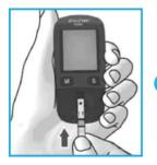
Take out one strip from the test strip box and carefully place it in its socket in the direction of the arrow without bending it.
